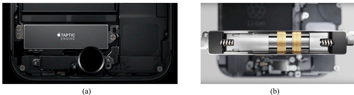
Figure 2. (a) Taptic Engine and the home button of an iPhone. (b) Vibration motor of an iPhone. From “Apples Taptic Engine: Entwickler können drei Modi nutzen,“ by Nicolas 2016. Retrieved from https://www.iphoneticker.de/apples-taptic-engine-entwickler-koennen-drei-modi-nutzen-102452/
