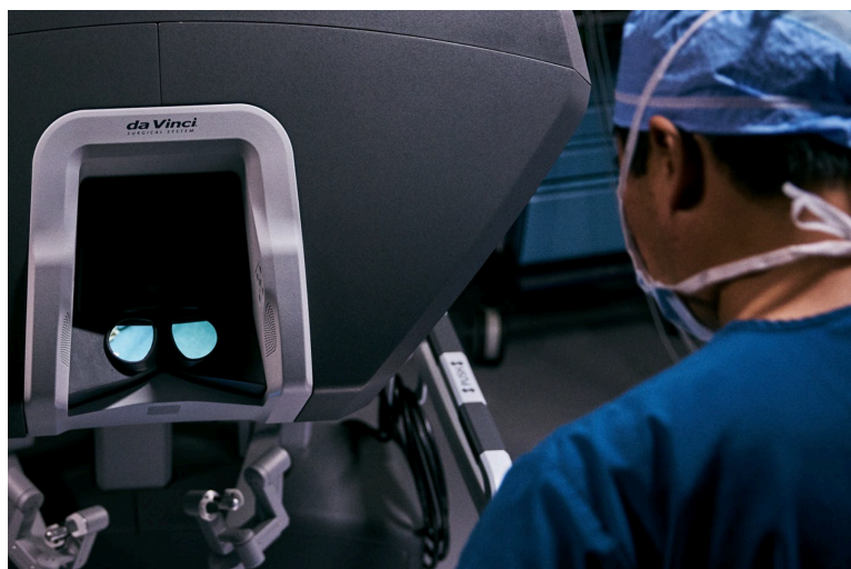
Figure 1. The da Vinci XI surgeon console with a look at 3D high-definition stereo viewer. From Intuitive, n.d. Retrieved from https://www.intuitive.com/en-us/products-and-services/da-vinci/systems##
