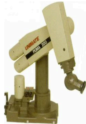
Figure 5. The programmable universal machine for assembly From “30 years of robotic surgery.” by Ghezzi & Corleta, 2016, World journal of surgery, 40(10), 2550–2557.
