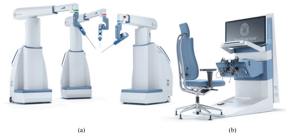
Figure 8. (a) Senhance patient cart (b) Senhance surgeon console. From Senhance, n.d. Retrieved with permission from https://www.senhance.com/us/digital-laparoscopy#senhance-system
