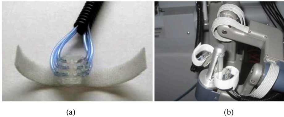
Figure 11. (a) Pneumatic actuator. (b) Pneumatic actuators mounted onto the da Vinci controls. From “Evaluating tactile feedback in robotic surgery for potential clinical application using an animal model.” by Wottawa et al., 2016, Surgical endoscopy , 30(8), 3198–3209.
